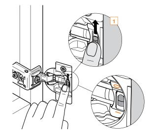
Door must be closed once for the deactivation to be complete. To reactivate, move switch back to the original position "I".
