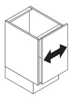
**Side Adjustment** Rotate the front cam screw to increase or decrease door overlay (+/- 1/16").
