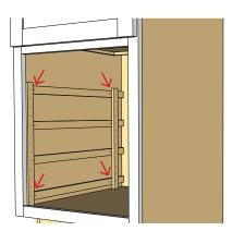
3. Install Blum® clips on underside of drawer box
